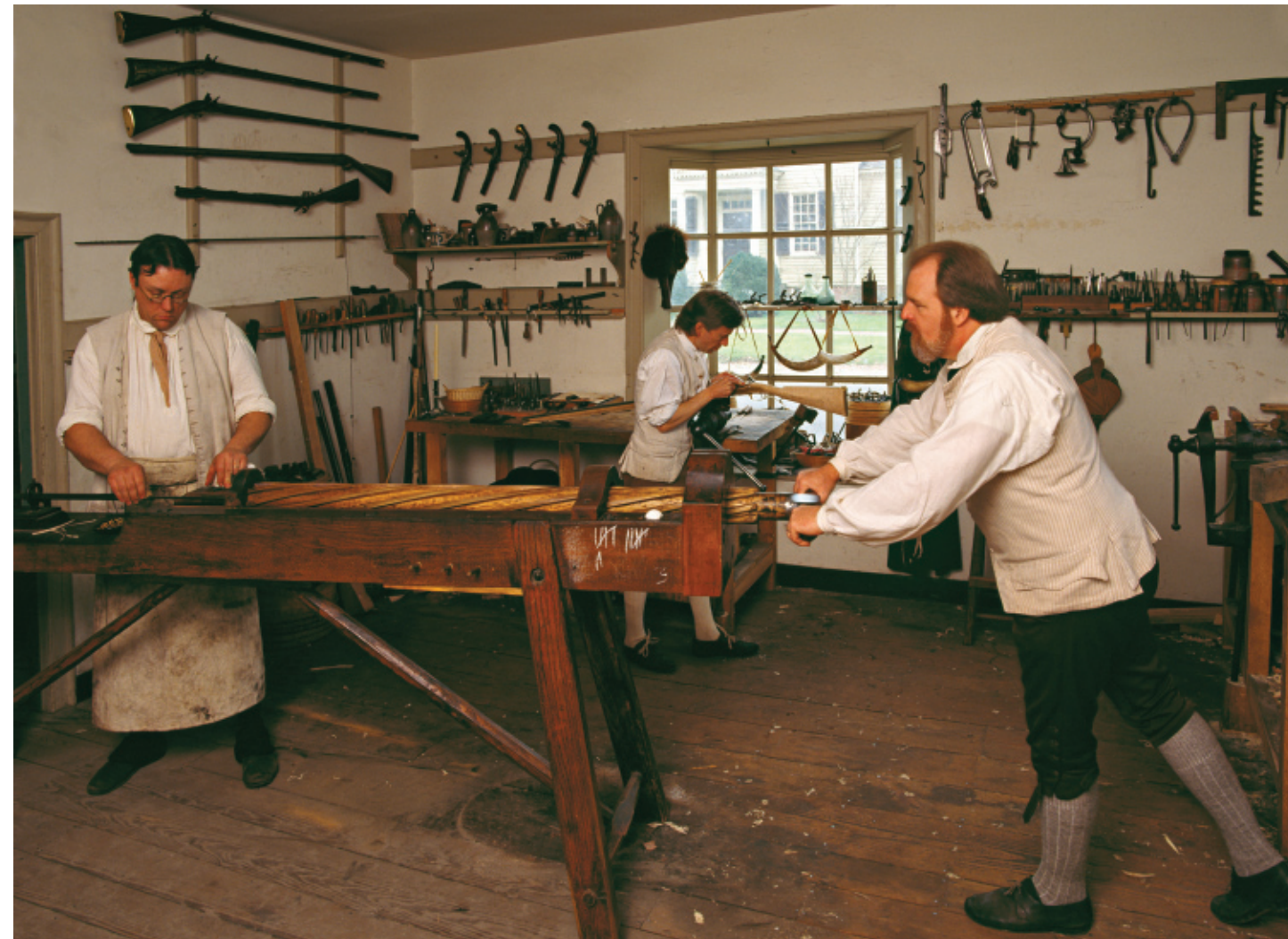
Below: Current Gun Shop Master George Suiter (r) rifling a hand forged gun barrel with journeyman Clay Smith assisting, while journeyman Richard Frazier works on a lock.
